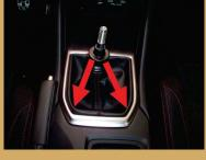
Remove the bolts securing the center console.
