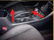
Remove the parking brake cover. Remove
