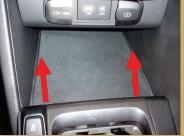
Remove the screws securing the center console.
