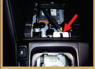
Remove the screw holding the trim under the steering column.
