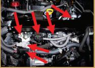
Disconnect the vacuum valve plug and remove the valve.
